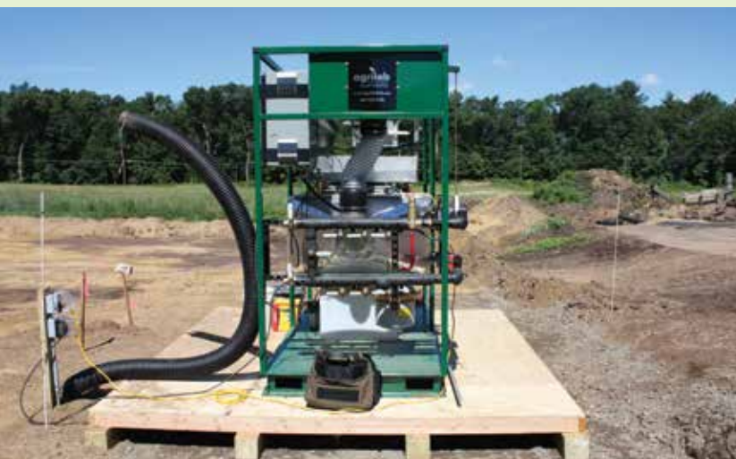
At left: the Agrilab Technologies Hot Skid 250-R consists of the mechanical aeration, heat recovery, plumbing, monitoring and control components.
